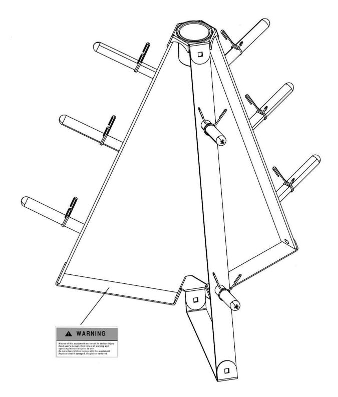
The Warning Label shown here has been placed on the Base Frame. If the label is missing or illegible, please call customer service at 1-800-999-8899 for replacement. Apply the label in location shown.
